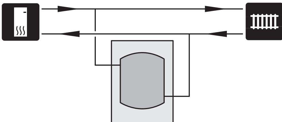
A UKV 100 is installed as a volume and flow increaser in those cases where the system volume in the climate system is below the minimum recommended volume for the heat pump and/or the flow is restricted without control.
