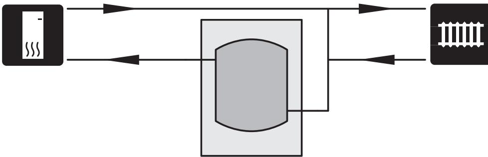
A UKV 100 is installed as a volume increaser in those cases where the system volume in the climate system is below the minimum recommended volume for the heat pump.
