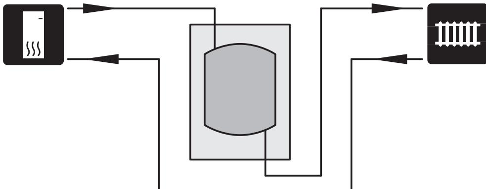
A UKV 100 is installed as a volume increaser in those cases where the system volume in the climate system is below the minimum recommended volume for the heat pump.
