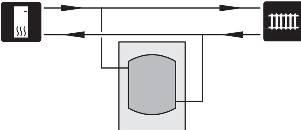
A UKV 40 is installed as a volume and flow increaser in those cases where the system volume in the climate system is below the minimum recommended volume for the heat pump and/or the flow is restricted without control.
