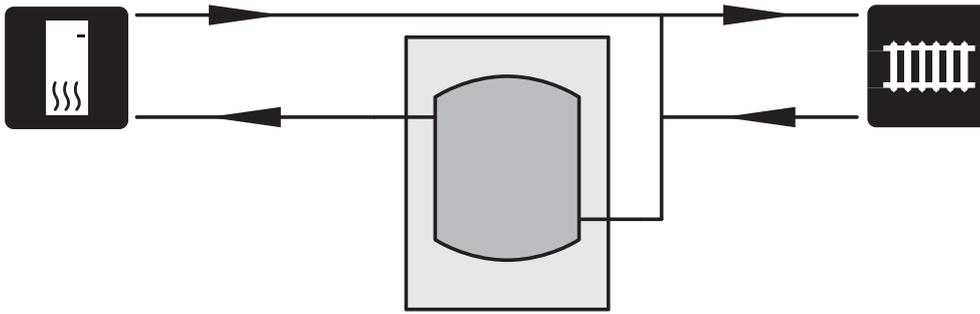
A UKV 40 is installed as a volume increaser in those cases where the system volume in the climate system is below the minimum recommended volume for the heat pump.
