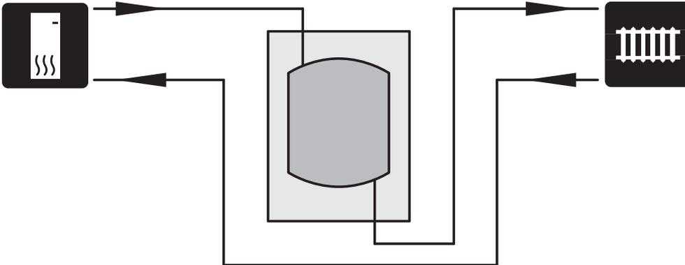
A UKV 40 is installed as a volume increaser in those cases where the system volume in the climate system is below the minimum recommended volume for the heat pump.
